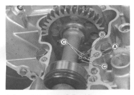
A. Crankshaft Gear C. Punch Mark
