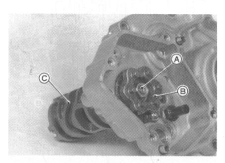
A. Mounting Bolt B. Pin Plate
