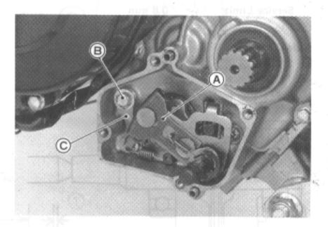
A. External Shift Mechanism C. Positioning Lever
